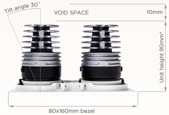
**\*Low void option available to give a unit height of 76mm. 2x Ø72mm cut out (80mm centres).**
